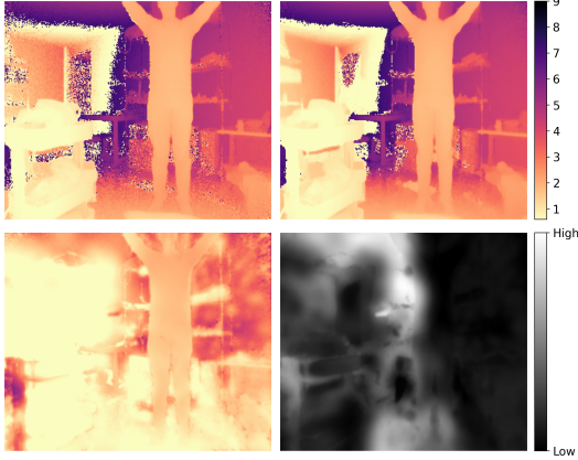
Figure 2. Fitting ToF Images \neq Fitting Depth. Top left: Camera-derived depth from C-ToF. Top right: Rendering a GS scene reconstruction into C-ToF raw images samples, then deriving depth. As this is similar to the camera-derived depth to the left, the reconstruction objective was met. Bottom left: Rendered mean scene depth from Gaussians, which is highly inaccurate. Bottom right: Depth distortion error [9], which measures the Gaussian sparsity along each ray. Gaussians are not well localized.
